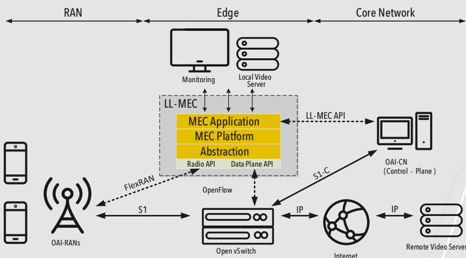
LL-MEC enables versatile applications, such as radio-aware video content optimization. It can adjust video quality based on the real-time per-user wireless channel quality to reduce the video stalling and to utilize all available radio resources. For instance, a user with poor channel condition only receives a 240p video, while another one can benefit from 4K video streaming when it is close to the base station.
